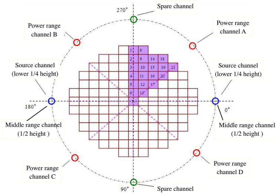
Fig. 1. Arrangement diagram of the PWR's ex-core nuclear measurement system.
