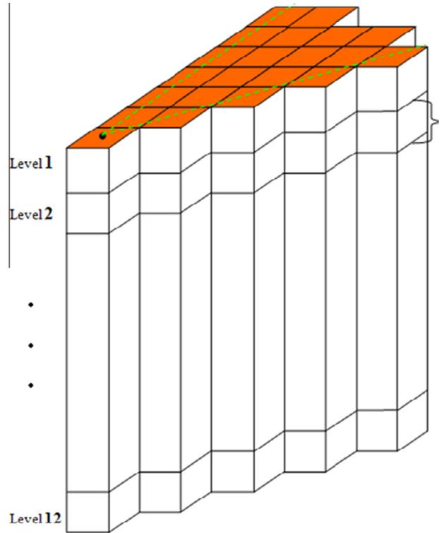
Fig. 2. The partition diagram of 3D reactor core segment.
