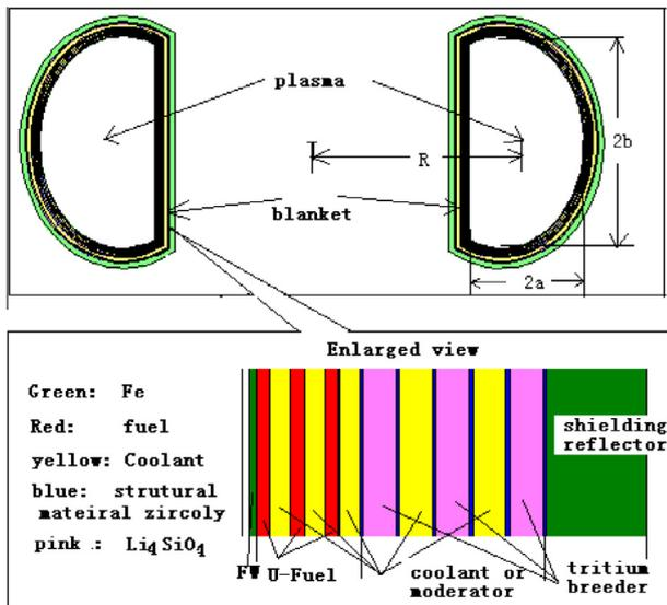
Fig. 1. Computational ‘D-Shape’ model of water cooled natural uranium/thorium fueled FFHR.
