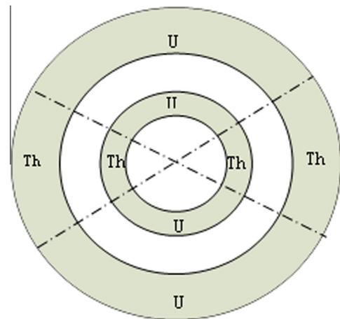
Fig. 2. Alternately arrangements of natural uranium and thorium modules in the toroidal directions of the blanket (equatorial plane).
