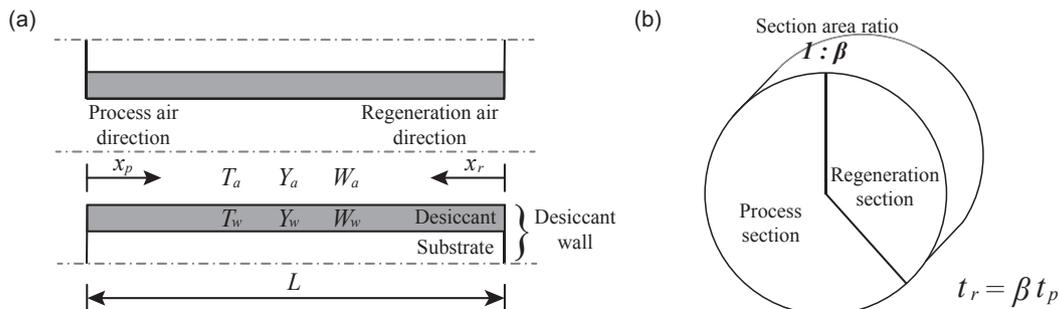
Fig. 1. (a) Schematic diagram of the channel of desiccant wheels (b) illustration of a desiccant wheel in which the split ratio between process area and regeneration area is set as 1:β.
