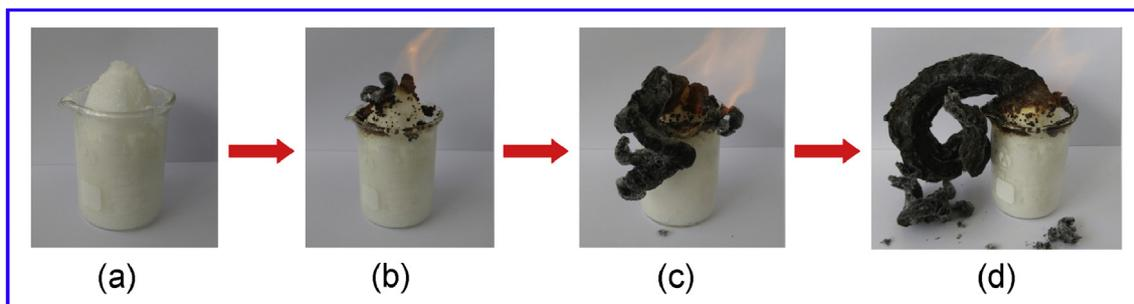
Fig. 1. Synthesis process of porous carbon foam by combustion reaction.
