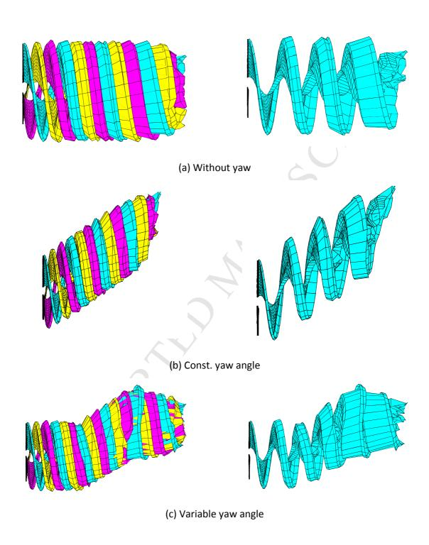
Wake structure behind the rotor at different yawed conditions from three blade (Left)
