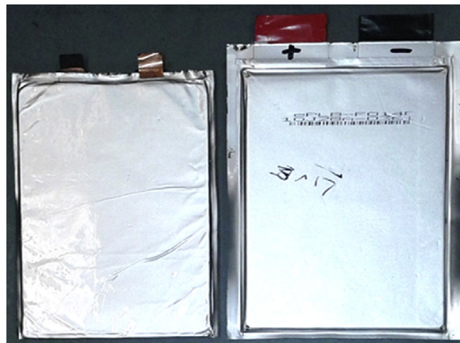
Fig. 1. Image of the 10 Ah LFP cell (left) and 14.5 Ah LFP cell (right).
