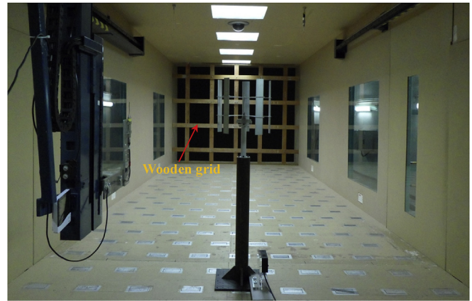
Fig. 1. Five-straight-bladed VAWT in the wind tunnel.
