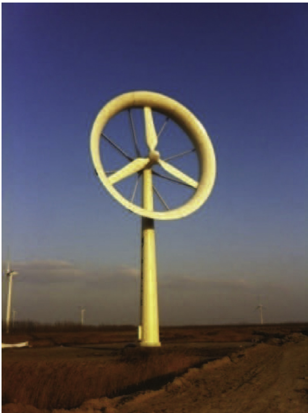
Fig. 1. A 200 kW wind turbine with compact wind lens (The photo is provided by Aviation Power Control Co., Ltd in China).
