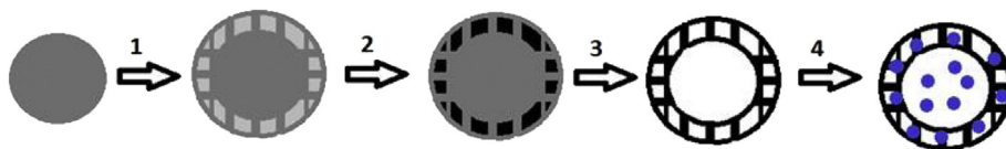
Fig. 1. Synthesis schematic of hollow carbon spheres (black) decorated with metal oxide nanoparticles (blue). Mesoporous silica spheres (grey) are being carbonized (step 2). After removal of silica (step 3), the resulting hollow carbon sphere is functionalized by metal oxide nanoparticles (step 4). (See the text.) (For interpretation of the references to colour in this figure legend, the reader is referred to the web version of this article.)
