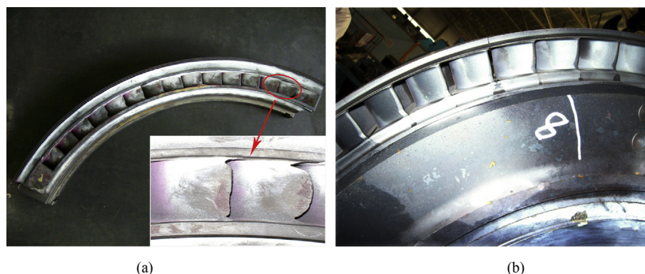
Fig. 1. Erosion morphology of control stage blades in a supercritical steam turbine: (a) Erosion of control stage nozzle; (b) Erosion of control stage rotating blades.
