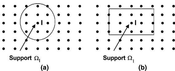
Fig. 1. The commonly used supports of node I: (a) circular and (b) rectangular.
