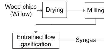
**Fig. 2.** Simplified flow sheet of syngas production from willow without torrefaction. Note: Untreated willow is assumed to be able to be gasified in an entrained flow gasifier. Moreover, the same gasification conditions as those used for torrefied wood are assumed applicable.
