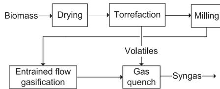
**Fig. 1.** Simplified flow sheet showing the idea behind integrated torrefaction as presented in Ref. [4]. Note: for case c and d presented in the text: biomass = wood chips (willow).
