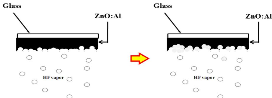
**Fig. 2.** The schematic diagram of vapor texturing process.
