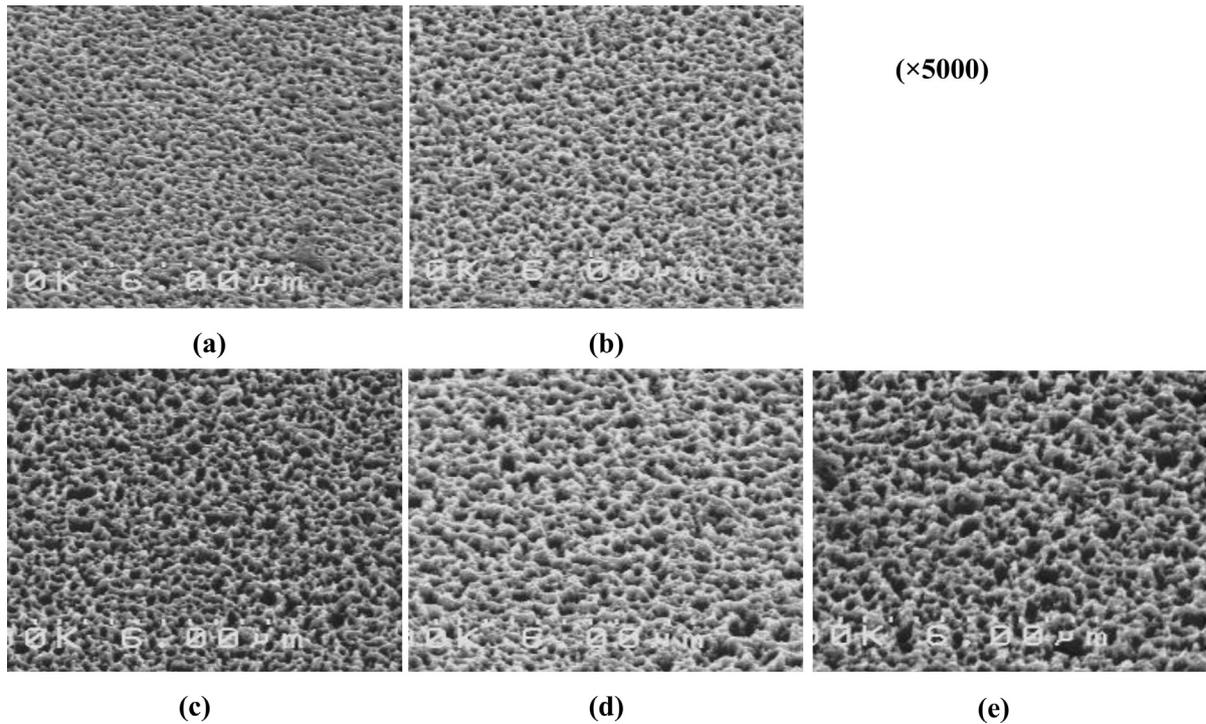
**Fig. 1.** Surface images of ZnO:Al films after HF vapor texturing under different conditions by FE-SEM. (a) sample A, (b) sample B, (c) sample C, (d) sample D, and (e) sample E).
