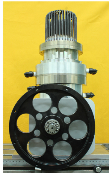
Fig. 1. Schematic and photo of 300-W beta-type Stirling engine with rhombic-drive mechanism [Model NCKU300-2, developed by Power Engines and Clean Energy Laboratory (PEACE Lab.), National Cheng Kung University].
