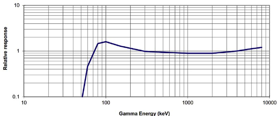
Fig. 1. HPIC relative efficiency with respect to photon energy (GE Energy, 2008).
