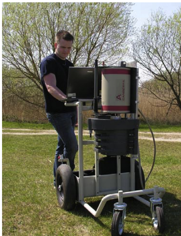
Fig. 1. HPGe detector with shielding system on a transport trolley, during measurement of in situ soil surface.
