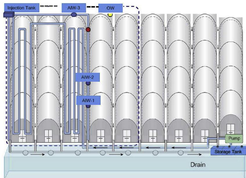
Fig. 1. Schematic diagram and positions of the three abstraction-injection wells (AIW) and one observation well (OW)\*. Sand filtration units were placed in front of the storage tank.
