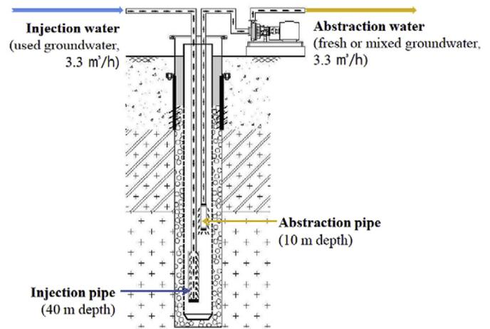
Fig. 2. Structure of the combined abstraction-injection wells constructed at the study site.
