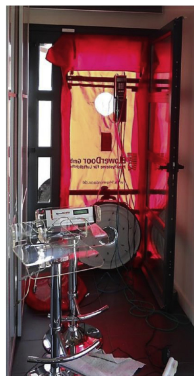
Fig. 2. Blower Door installation and continuous indoor radon measurement.
