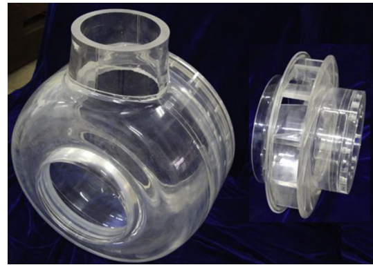
Fig. 2. The transparent plexiglass casing and diffuser.
