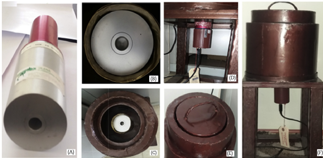
Fig. 1. Setup gamma ray spectrometer, (A) The 3" × 3" well-type NaI(Tl) detector with photomultipliers, (B) Cu layers, (C) The opening for samples changing, (D) The photomultipliers passing through the lower part of the shield, (E) Cover shield, (F) The assembled shield.
