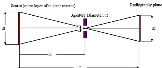
Fig. 1. Schematic view of the designed radiography system.
