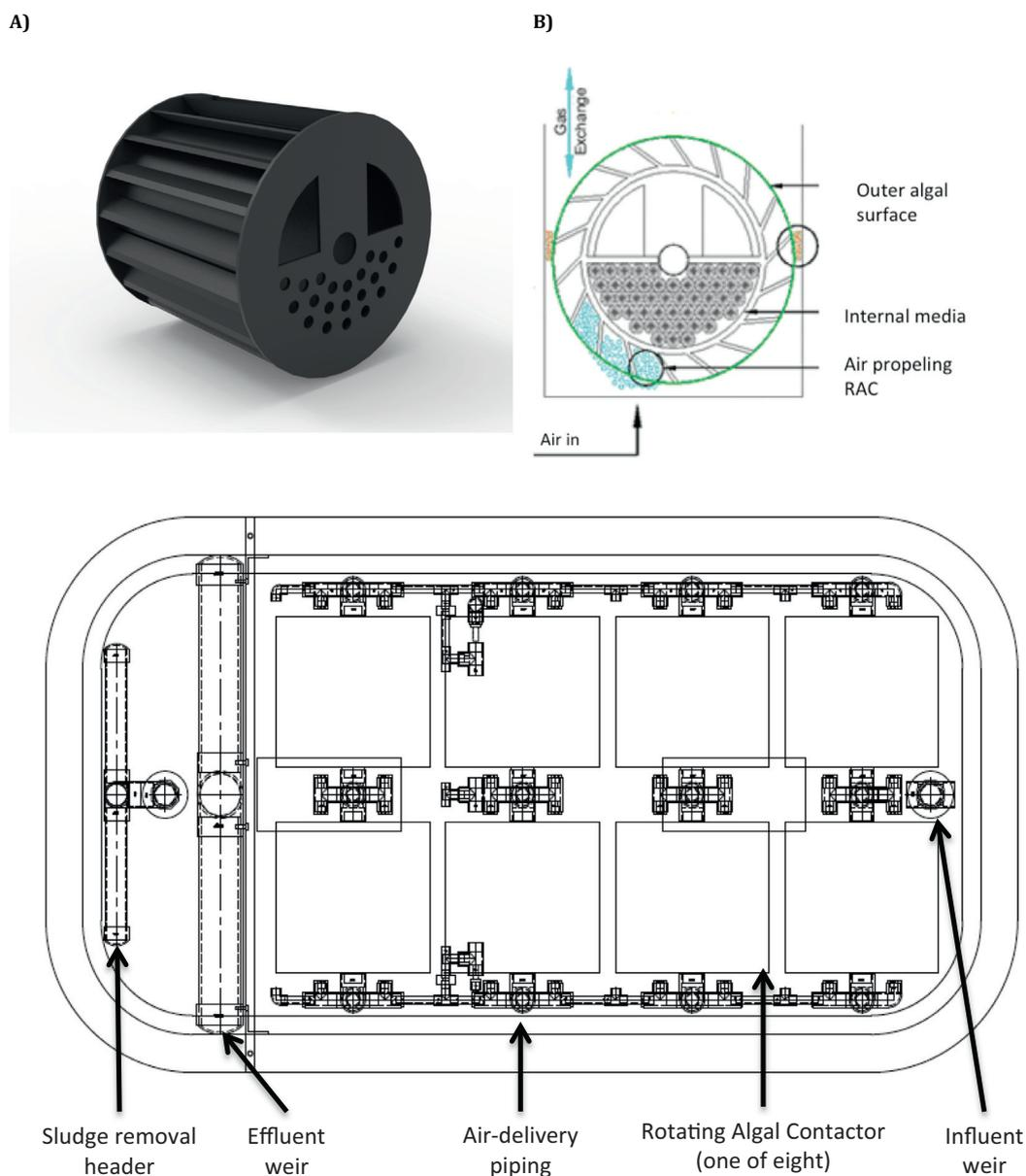
**Fig. 1.** Reactor components and layout. A) Algaewheel™ rotating algal contactor (RAC), B) RAC showing interactions with air bubbles and water, C) plan view of the reactor/tank (2.43 m × 1.2 m × 0.25 m).
