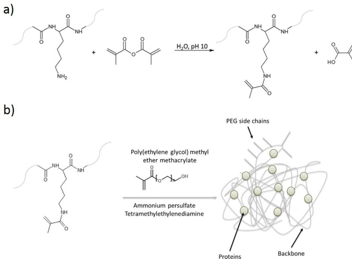
Fig. 1. Two-step reaction for synthesizing polyurethane-like elastomers: a) methacrylation of proteins, b) co-polymerization with PEGMA in the presence of APS and TEMED.
