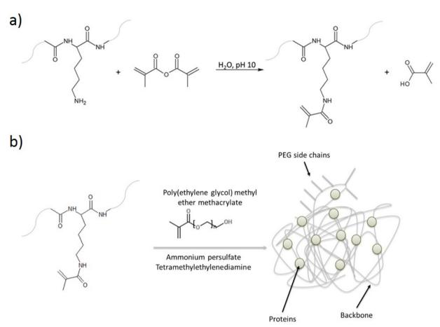
Fig. 1. Two-step reaction for synthesizing polyurethane-like elastomers: a) methacrylation of proteins, b) co-polymerization with PEGMA in the presence of AMPS and TEMED.
