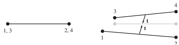
Fig. 1. Line interface element in an initial (left) and deformed (right) configuration.
