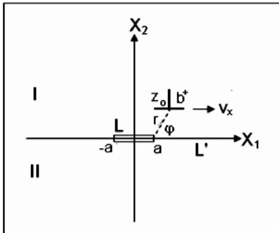
Fig. 1. A moving screw dislocation near an interfacial crack in two orthotropic media.
