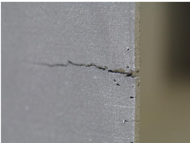
Fig. 1. Failure during manufacturing of a Ti-6Al-4V component caused by the build-up of residual stress.
