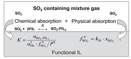
Fig. 1. The mechanism of SO<sub>2</sub> capture by functional ILs (Reprinted with permission from Ref. [7]. Copyright (2011) American Chemical Society.).
