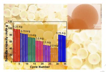
Self-supported carbon nanospheres are prepared by a facile hydrothermal method and demonstrated with good sodium ion storage performance
