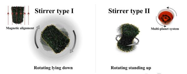
Two distinctive RGO-Fe<sub>3</sub>O<sub>4</sub> stirrers were achieved that could dynamically respond to the rapidly changing magnetic field while executing designed movements precisely: rotating with lying down posture or standing straight posture, which demonstrates bright prospects in energy and environmental applications.
