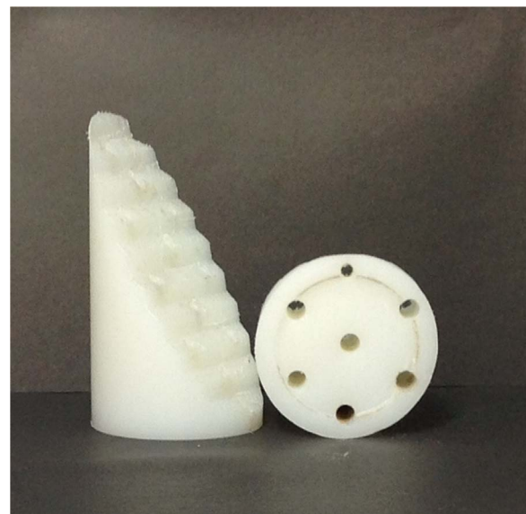
Fig. 1. Polyethylene specimen used as the rock fracture specimens.
