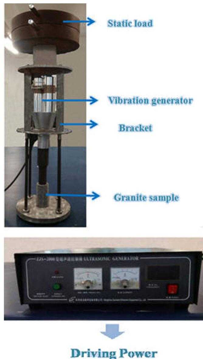
Fig. 1. Photographs of the special ZJS-2000 ultrasonic vibration device.
