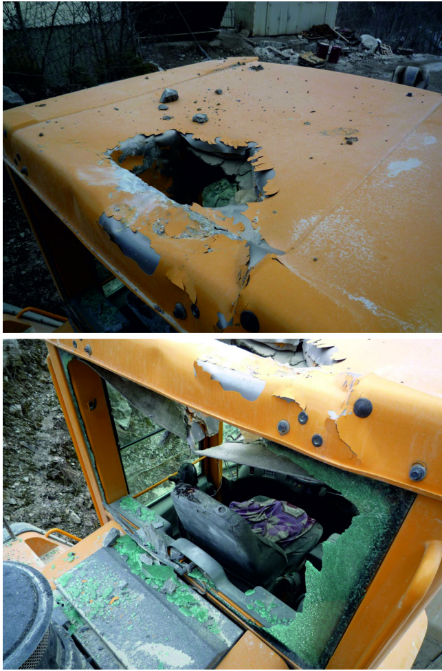
Fig. 1. Photo of a rock fall accident at a quarry in Austria.
