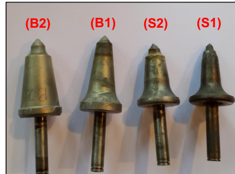
Fig. 3. Four cutting tools tested for frictional ignition. B1, BETEK coal cutting bit; B2, BETEK rock cutting bit; S1, Sandvik coal cutting bit; S2, Sandvik rock cutting bit.
