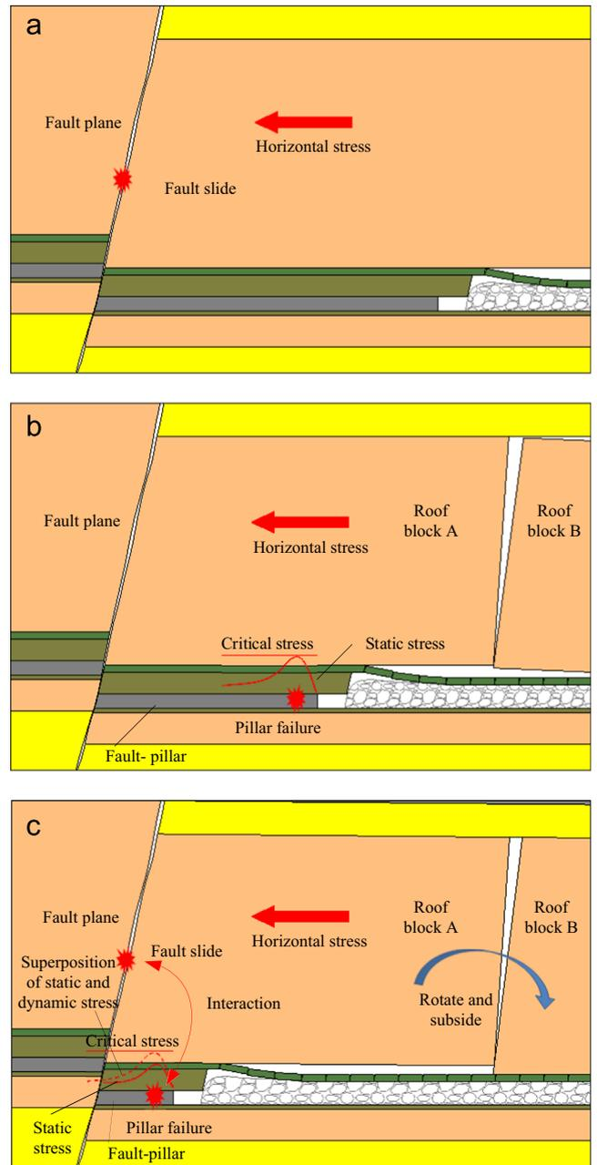
Fig. 2. Sketches showing the mechanism associated with FPIRB.
