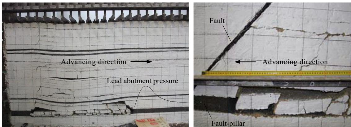
Fig. 1. Strata movement characteristics probed using physical simulation.
