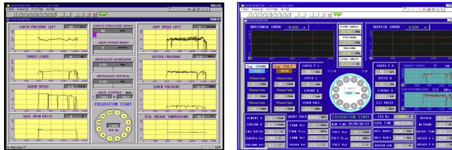
Fig. 1. TBM control cabin main display screens showing excavation data and machine mechanical behaviour against the excavated material.
