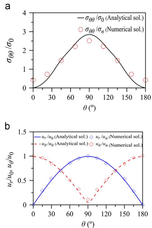
**Fig. 2.** Verification of the numerical model. (a) Normalized seismically induced stress increments in the tangential direction ( $\sigma_{\theta\theta}/\sigma_n$ ) obtained by numerical simulation and Pao's analytical solution [20], and (b) seismically induced displacements along a tunnel wall obtained by numerical simulation and Mow's analytical solution [21].
