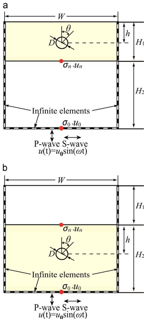
**Fig. 1.** Configurations of numerical models. (a) The tunnel is located in the upper rock layer, and (b) the tunnel is located in the lower rock layer.
