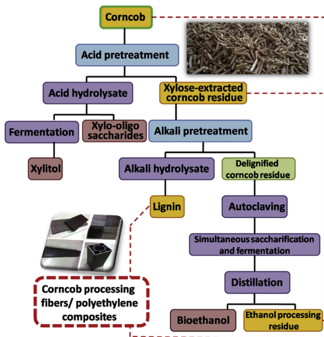
Fig. 1. Flow chart of the corncob biorefinery process. Solid fractions of CCB, X-ER and EPR in different pretreatment stages were used as the reinforcing phase of the WPCs.
