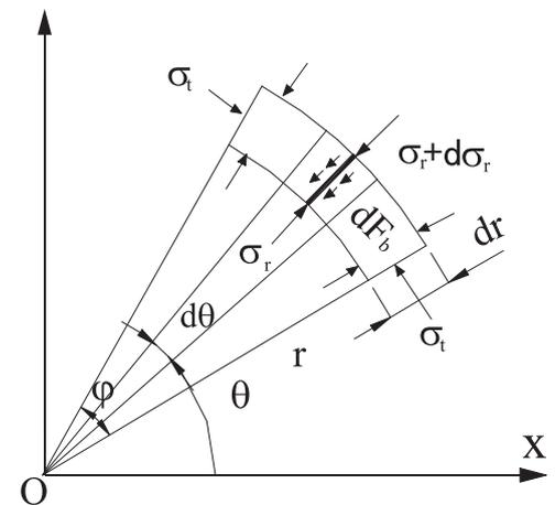
Fig. 3. Mechanical behavior of reinforced element.
