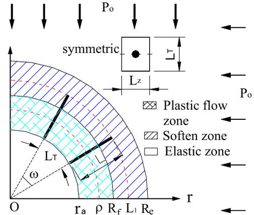
Fig. 1. Relative position of the rock bolt around tunnel.
