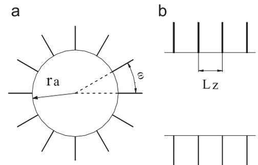
Fig. 2. Illustration of the rock bolting arrangement in tunneling.
