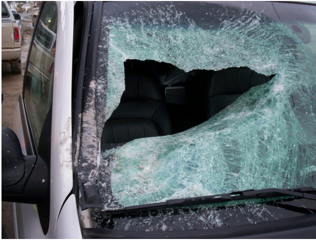
Fig. 1. Moving vehicle struck rock fall that passed through the windshield.
