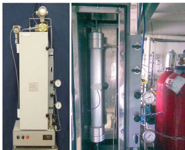
Fig. 1. Image of the gas separation membrane system (left-hand side) with the PI membrane module installed (right-hand side).
