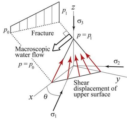
**Fig. 1.** Direction of shear displacement in a fracture in comparison with that of macroscopic water flow.
