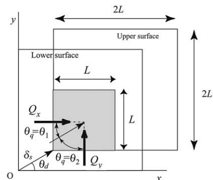
**Fig. 2.** Direction of shear displacement ( $\delta_s$ ) and the angle ( $\theta_q$ ) between the directions of shear displacement and macroscopic water flow ( $Q_x$  and  $Q_y$ ).
