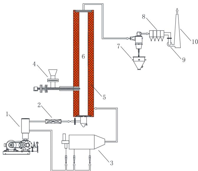
**Fig. 1.** Schematic diagram of the fluidized bed device. 1-air fan; 2-heat exchanger; 3-diesel combustion chamber; 4-hopper; 5- heating jacket; 6-fluidized bed reactor; 7-cyclone; 8-bag filter; 9-induced draft fan; 10-chimney.
