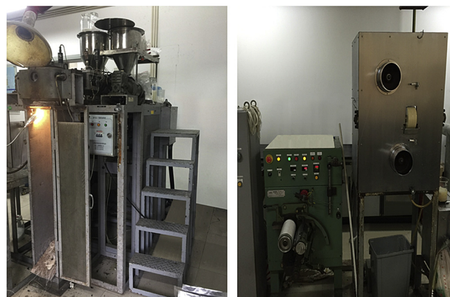
Fig. 1. MATE-V melt spinning device. Left: the extrusion portion; Right: the fiber winding portion.
