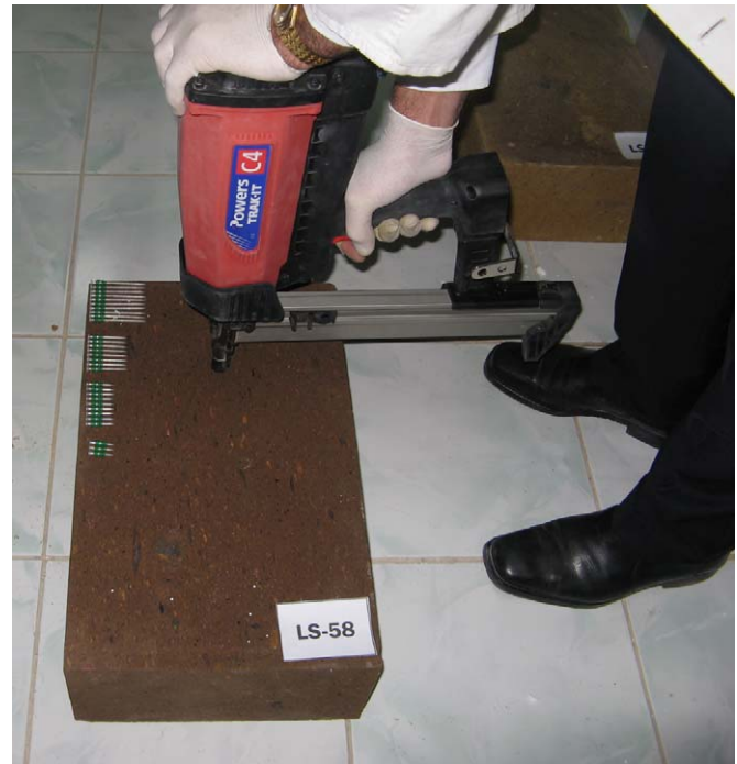
Fig. 1. The concrete nailer and the nail cartridges utilized in the investigation.
