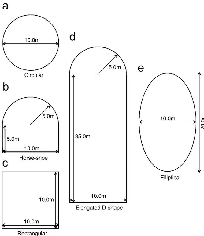
Fig. 1. Five different shapes of underground openings considered for analysis.
