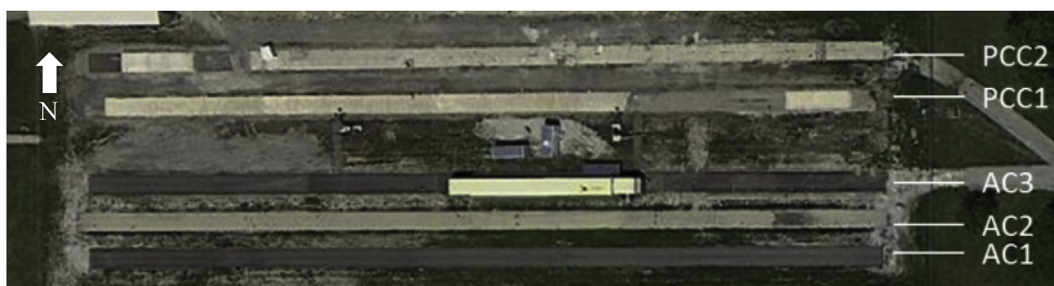
Fig. 1. Google Earth™ screenshot of the ATLAS facility with the five sections under study labeled AC 1–3 and PCC 1–2.
