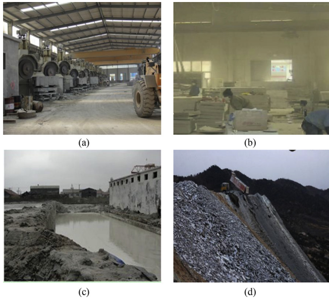
Fig. 1. The environmental issues caused by stone processing industry. (a) stone processing workshop (b) sawdust (c) wastewater (d) crushed slabs and scraps.
