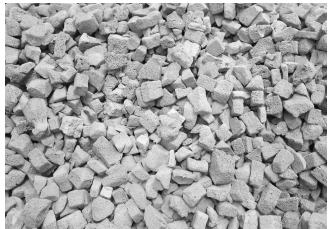
Fig. 1. Foamed recycled glass after production (courtesy of the Geotechnical laboratory at Swinburne University of Technology, Australia).
