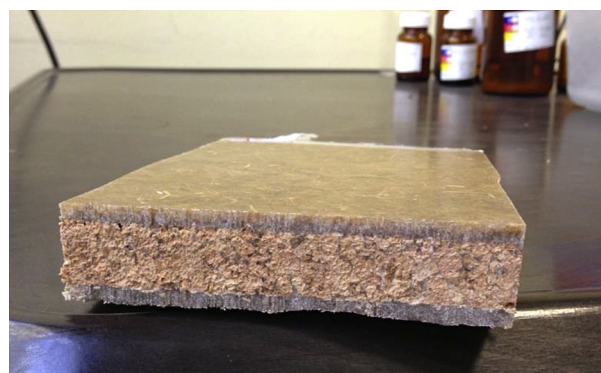
Fig. 1. Eco-sandwich with core in granulated cork and skins in hemp/bio-resin.
