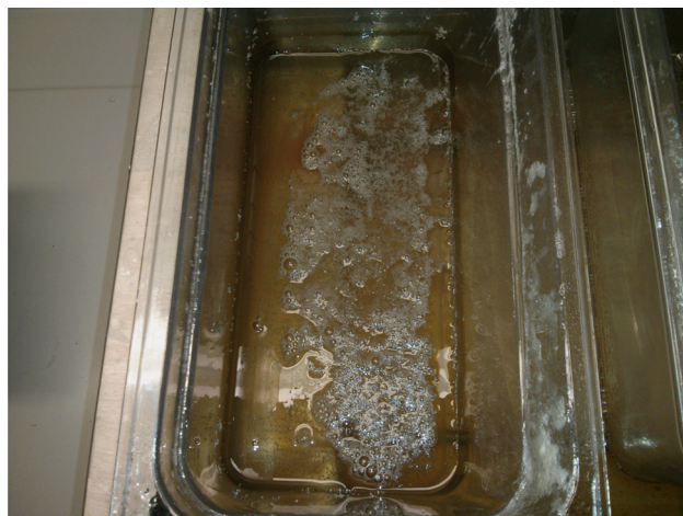
Fig. 1 – Liquid gelatin cast into the mould after dissolving the gelatin powder in water. Scum is visible on the top layer of the material.
